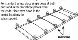
**Tip:** You can place single or twist bows in different slots to create a setup with custom support.
